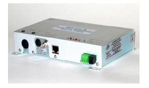
ECT055 system provides high performance link for transmitting RS-485 data signals over a fiber optic cable. The system supports 2 and 4 wire RS-485 interfacing and speed-independent RS-485 transmission.
