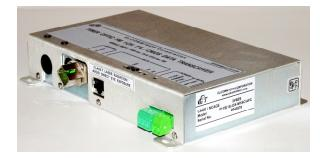
ECT002 system provides two duplex channel high performance link for bidirectional transmitting data signals over a fiber optic cable. The system features quality transmission of data signals with data rates DC - 10 Mb/sec.
