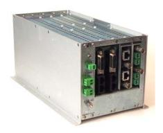
The USR-4D is a universal subrack designed for small and flexible integration projects. The subrack accepts all Elcommtech's card style products.
