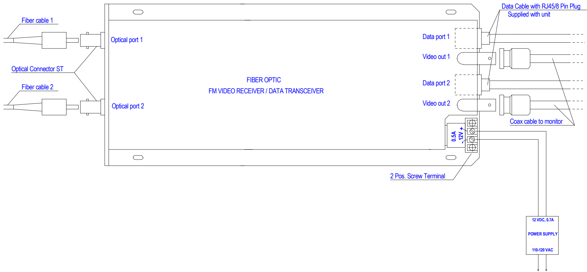
244S-VR/DX-M2 Video Receiver / Data Transceiver Connections Diagram
