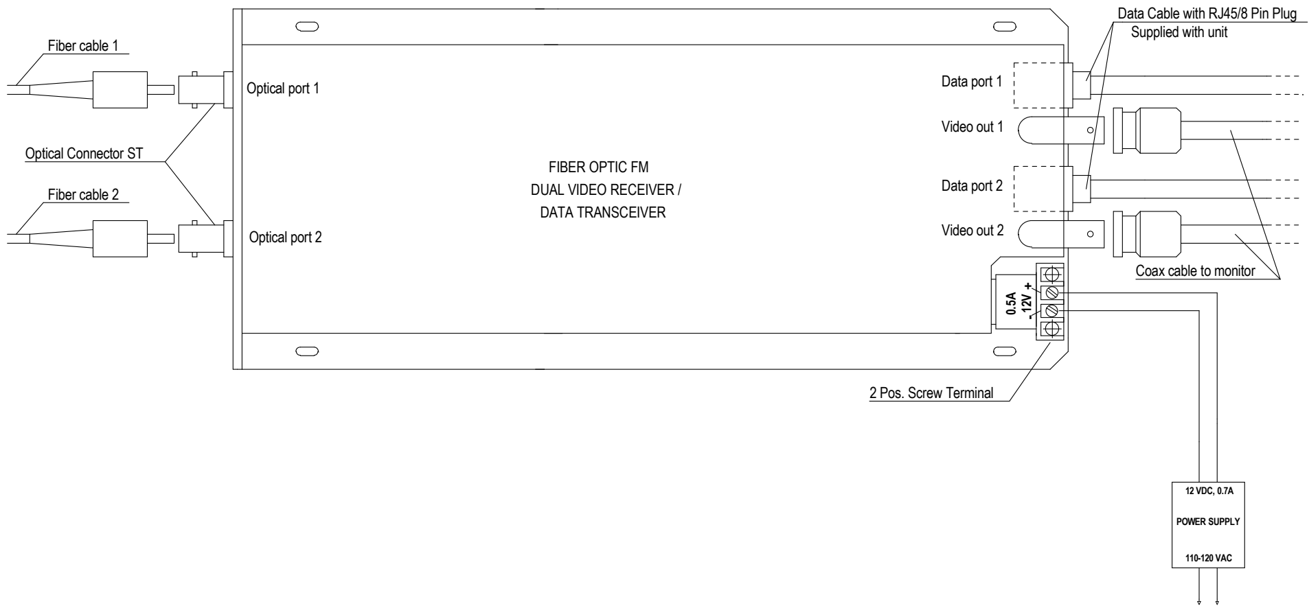
233S-VR/DX-M2 Video Receiver / Data Transceiver Connections Diagram
