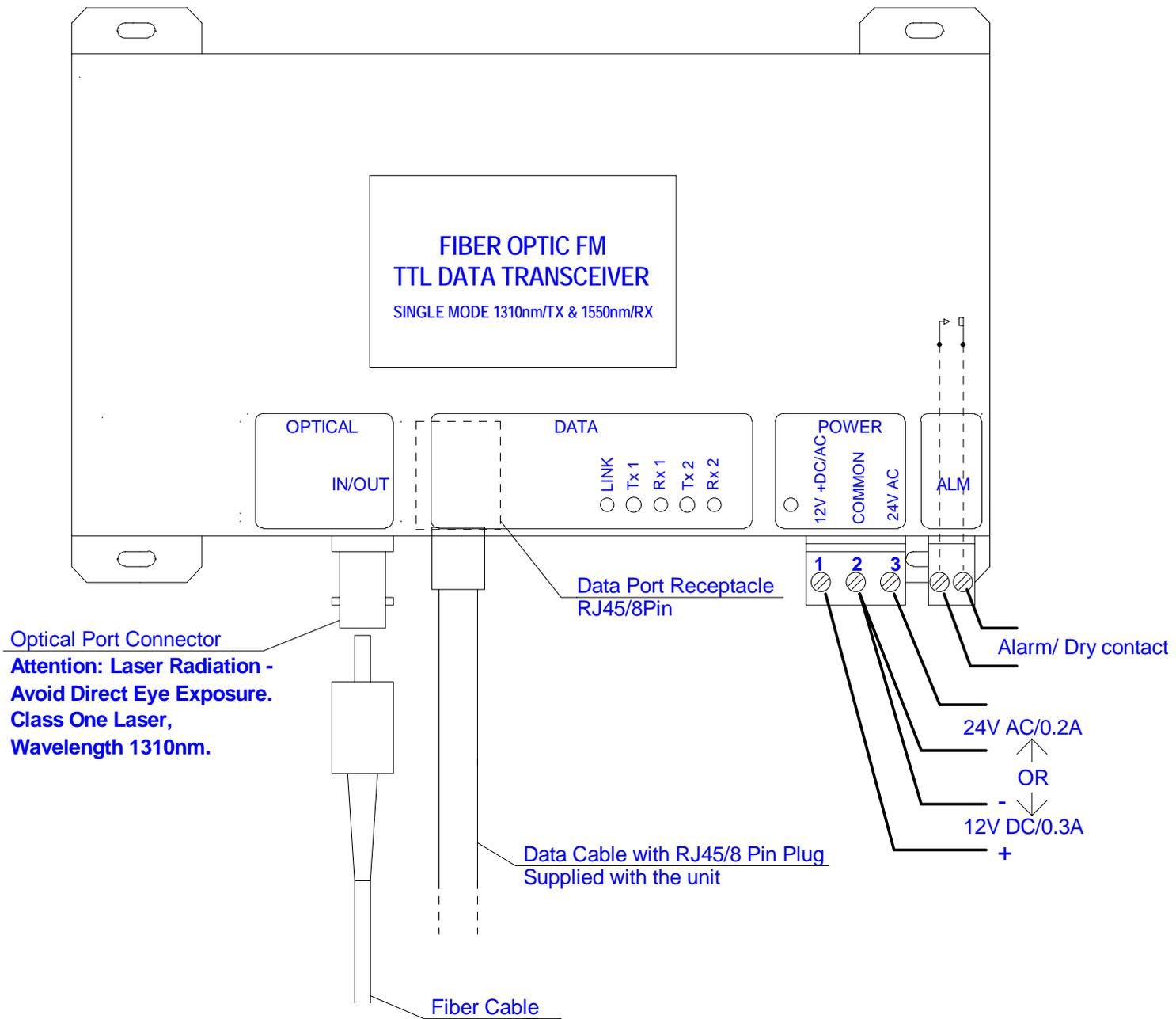
014S-DX2-M1ST TTL Data Transceiver Connections
